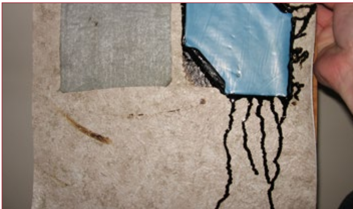
Compatibility is an important consideration in order to avoid messy situations like with this peel & stick membrane incompatibility.
