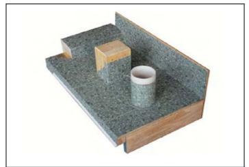
Curbs, knee walls, posts, and wall openings must be built and detailed to ensure membrane performance. In constructing or modifying door openings, door sills should be sloped toward the deck surface for optimum drainage, and the waterproof membrane should continue into the rough door opening saddle
