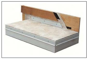
Although building papers do not cause an issue, asphaltic products (e.g. peel-and-stick membranes) must be separated from PVC membranes with metal flashing, asphalt-compatible modified thermoplastic membrane, or aluminum foil tape. On projects where the deck is to be used as a staging area for other trades, protective panels should be applied over the finished membrane.
