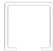
Glazing Channel Bottom Rail HEIGHT: 1" WIDTH: 1" ALLOY: 6063-T5
