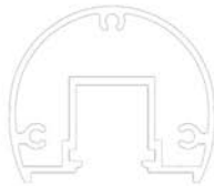
Durarail Round Top Rail (Component Glass) HEIGHT: 1 15/16" WIDTH: 2 1/4" ALLOY: 6063-T5
