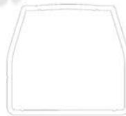
Component Glass Bottom Sleeve HEIGHT: 1 15/16" WIDTH: 1 1/2" ALLOY: 6063-T5
