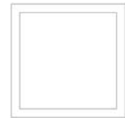
Fence Bottom Sleeve HEIGHT: 1 1/4" WIDTH: 1 1/4" ALLOY: 6063-T5
