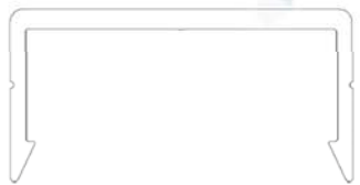
Welded Picket Bottom Rail HEIGHT: 5/8" WIDTH: 1 5/16" ALLOY: 6063-T5
