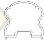
Durarail Heritage Top Rail (Welded Picket) HEIGHT: 1 15/16" WIDTH: 2" ALLOY: 6063-T5
