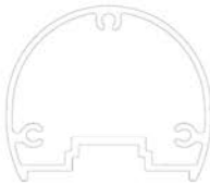
Durarail Round Top Rail (Welded Picket) HEIGHT: 2 5/32" WIDTH: 3 21/32" ALLOY: 6063-T5
