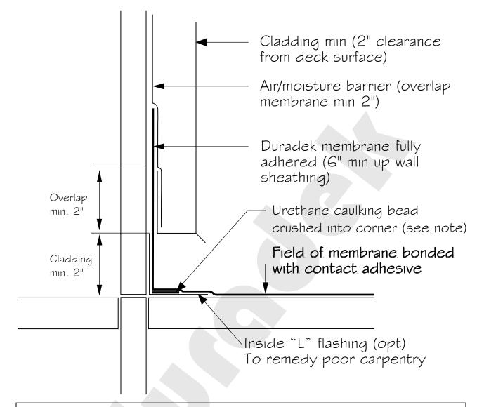
Note: This method requires the use of a bead of urethane cauking crushed into corner at the deck-to-wall transition.
