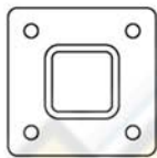
2"x2"x3/16" END POST WITH 4"x4"x1/2" BASE PLATE
