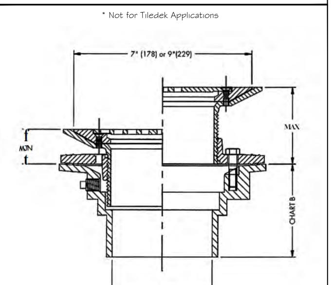
Note: Membrane clamped and caulked between strainer and body extension. We recommend the use of Watts FD-IOO-FC floor drain with surface membrane clamp for concrete deck applications.
